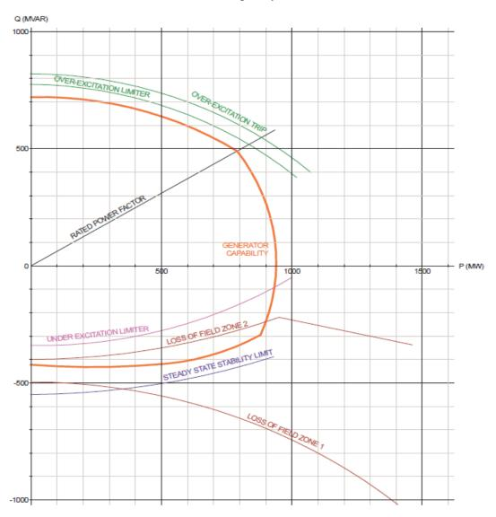
Section G Attachment 2 – Example of Capabilities, Limiters, and Protection on an R-X Diagram at nominal voltage and frequency
